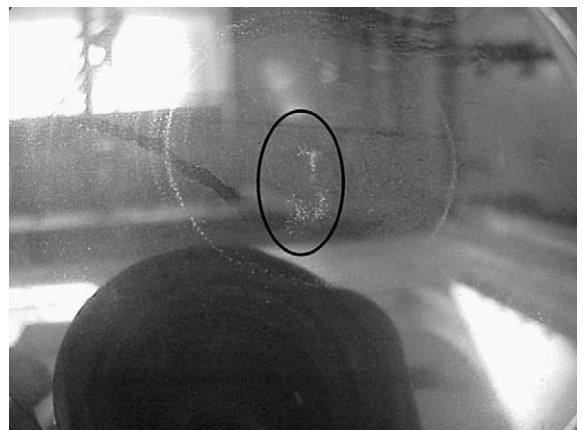
Fig. 9. Damage near the center of the front flange of LE3.
